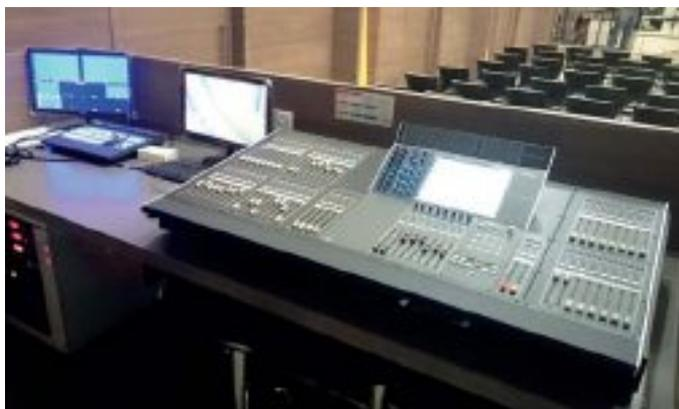
A Yamaha M7CL console at FOH has been inserted with an MY16A card for accepting the myMix monitor feeds
