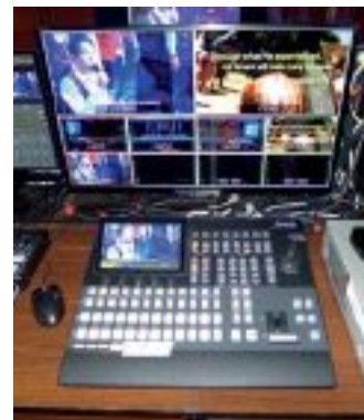
A Panasonic AV-HS410 switcher receives six feeds from Sony HD cameras and Apple Macs
