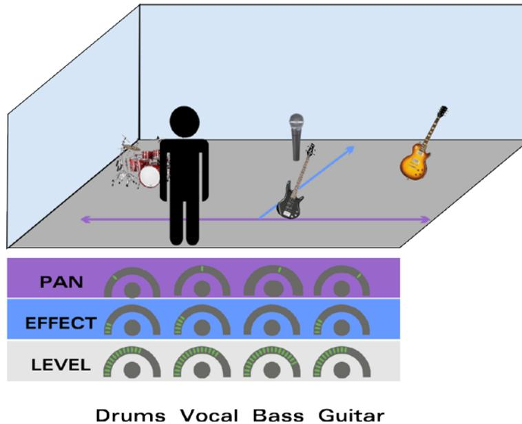
*Pic4: Adding more or less of effect for an instrument or a voice is like moving it more or less "deep" in the room. While PAN makes the left-right position, the amount of effect determines the "depth". The result is a 3-D sound image with clearly positioned sound sources.*
