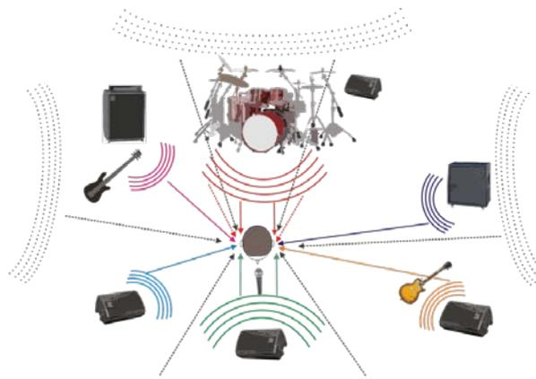
*Pic 1: on stage we hear the backline and monitor speakers as well as the reflections from the stage and the house pa system: a true 3-D sound image with localization and room information.*
