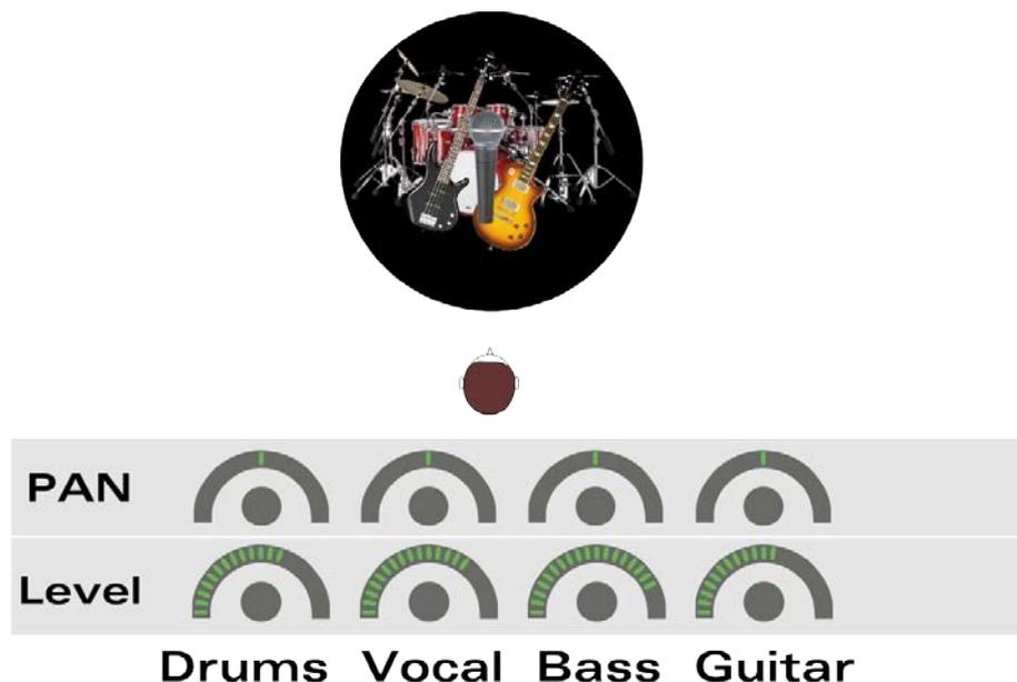
*Pic 2: a mono mix means feeding the exact same signal to both ears. This results in a one dimensional sound image with several consequences.*
