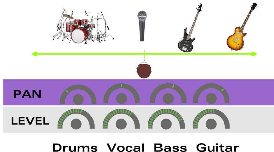
*Pic 3: using a stereo mix for the in-ear systems allows to position the signals within the stereo image. This helps the brain to differentiate them - a big improvement from the mono situation but still only a 2D sound image.*
